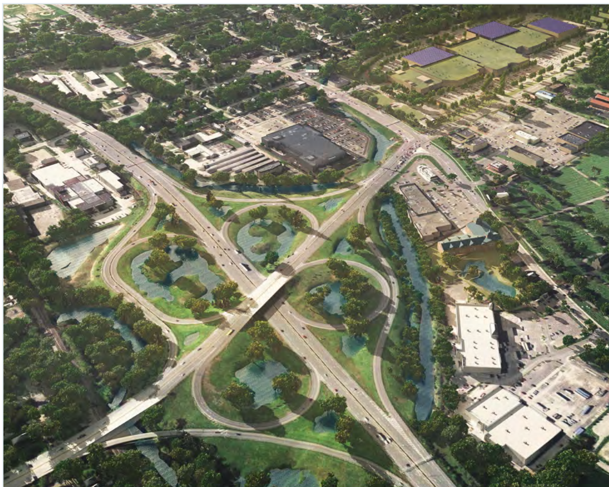
Pathways would allow floodwater to move freely between the four internal and smaller external segments of the cloverleaf.
